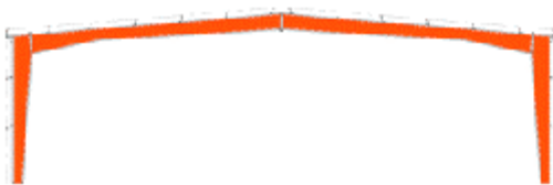
Gable Clear Span
