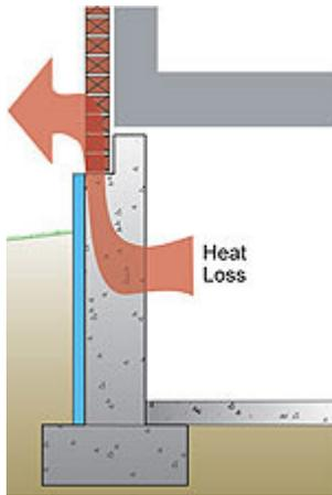
A thermal bridge is an assembly or component in the building envelope that transfers heat at a significantly higher rate than the surrounding insulated area. Fasteners, joints and gaps can create thermal bridging. It can cause significant heat loss or gain and underperformance of insulation assemblies in commercial buildings. Because IMPs use concealed fasteners and qualify as continuous insulation, thermal bridging is not a factor.
