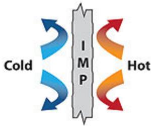
Continuous Air Barriers, also known as CABs, are special materials and/or assemblies that meet certain criteria for air infiltration as well as having all joints and penetrations sealed. By keeping the internal and external environments separate, CABs enhance energy efficiency and are required by newer energy efficiency building codes and standards.
